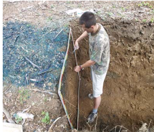
Fig. 4: Cleaning of soil profile by scissors.
